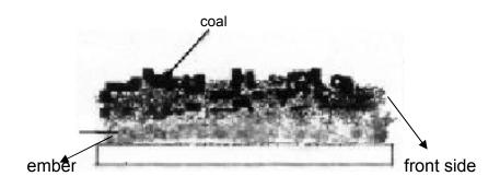
The coal must take as it's emble as the boiler spit at the under of it for to ignitate the boiler again in the morning. If the emble's quantity is low, by the help of some firewood adding, increase the emble quantity and the boiler must reload by the shape of loading platform.
